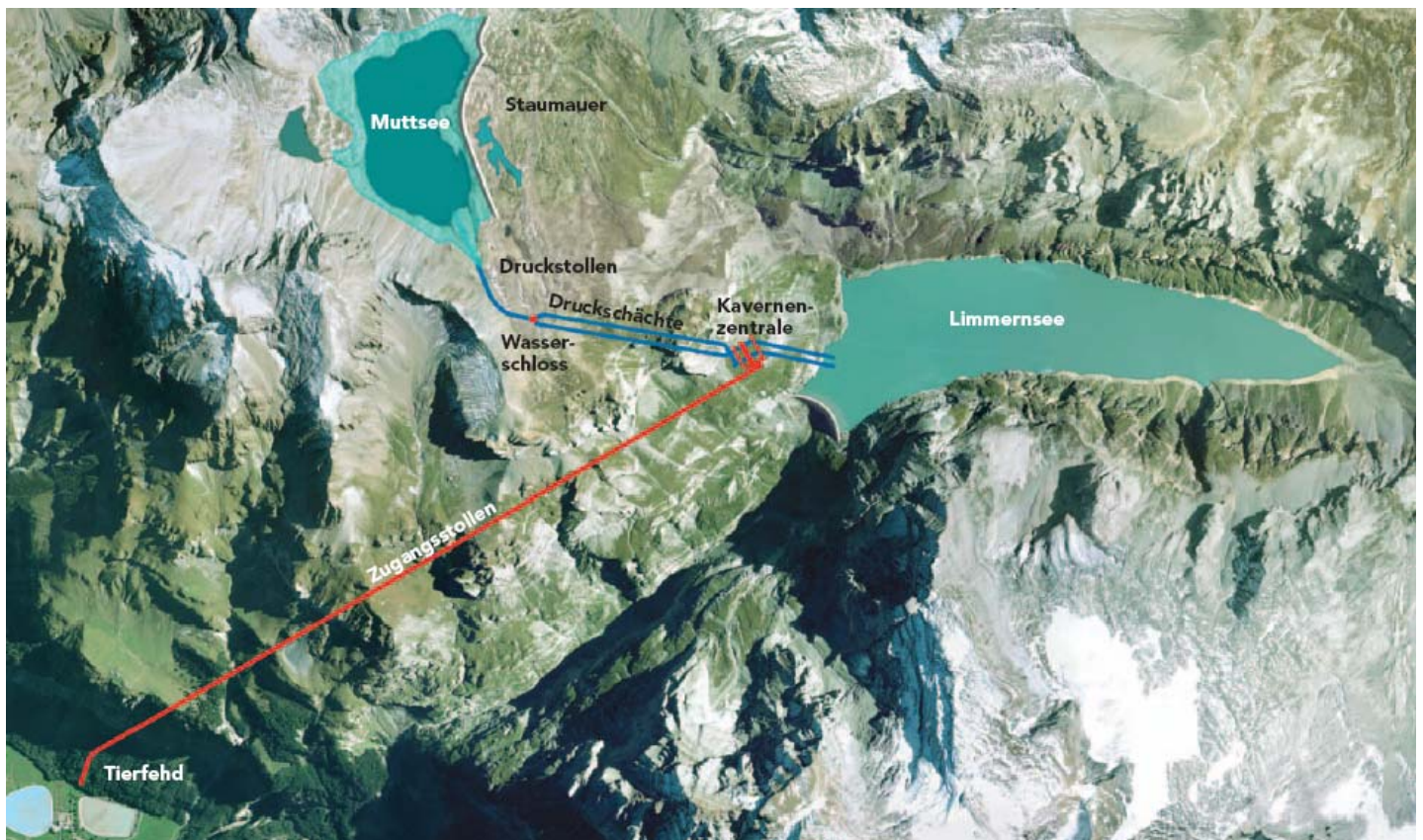
Figure 1. Situation of the plant between the lower reservoir lake Limmern and the upper reservoir lake Mutt.
