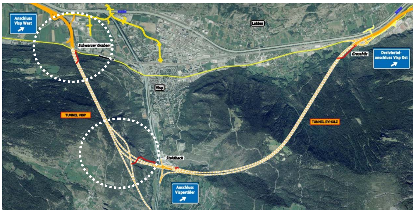
Figure 1. Situation of the Visp by-pass with underground junction (lower left) and portal "Schwarzer Graben" (upper left).
